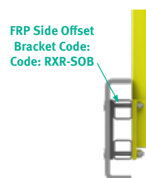
Side Off-Set Mounting to FRP/Steel*
