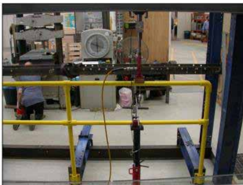
Figure: 2 Subject: Top rail point load vertical test with load cell at top hydraulics.
