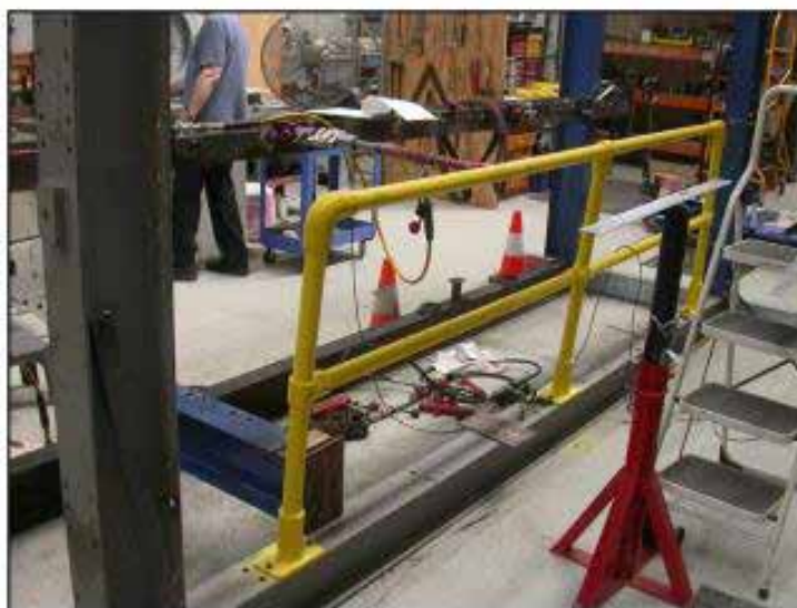
Figure: 1 Subject: F-RXH-R (1m high x 3m long) under the horizontal rail point load.
