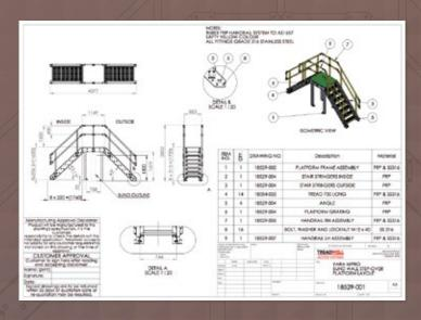
The ArchitEX™ Crossover System was designed and manufactured with corrosion resistant GratEX® FRP grating, RailEX® FRP handrails and a range of ArchitEX™ FRP structural profiles which are manufactured from premium grade fibreglass resins that was categorically specified to withstand the corrosive.
